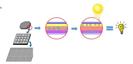
PV cells produce direct current (DC) electricity. Invertor's are needed to convert the DC voltage from the PV panel into alternating current (AC) voltage suitable for your home.
