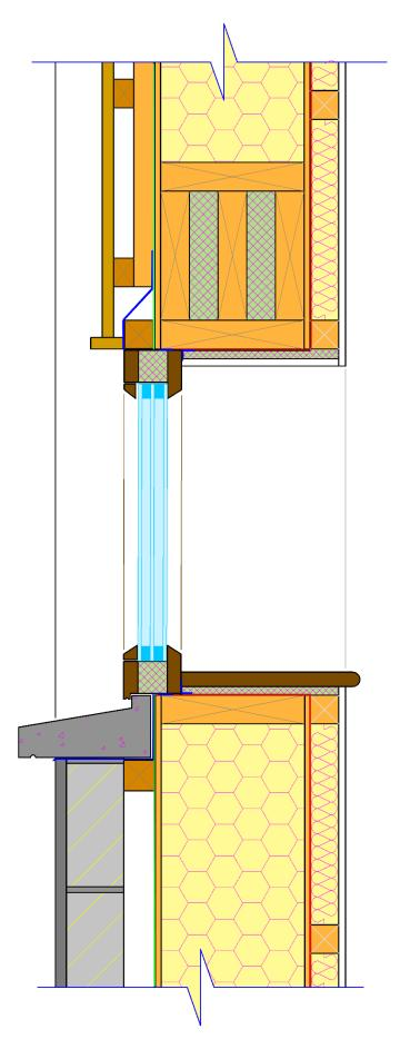
Typical best practice detailing of a fixed frame window and the external timber frame wall of the house
